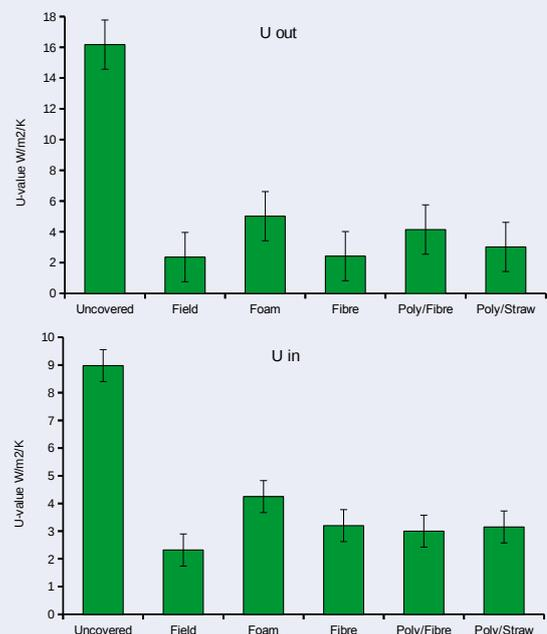
Measurement of soil temperature and moisture to a depth of 50 cm enabled calculation of hourly soil heat loss or gain and U-values (a standard measure of insulation, low = better). U out is for heat loss, U in is for heat gain.
